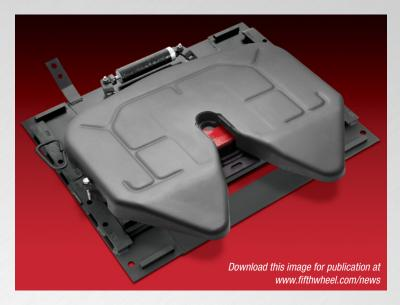
slide assembly. The net result is about 60 pounds lighter than the competition. Plus, you get the added benefit of running with Fontaine No-Slack® lock technology. The exclusive No-Slack® design automatically self-adjusts the lock to allow for trailer kingpin size variances. The precise No-Slack® kingpin fit reduces shock inputs into the frame for a smoother ride, lower maintenance costs and longer component life.
